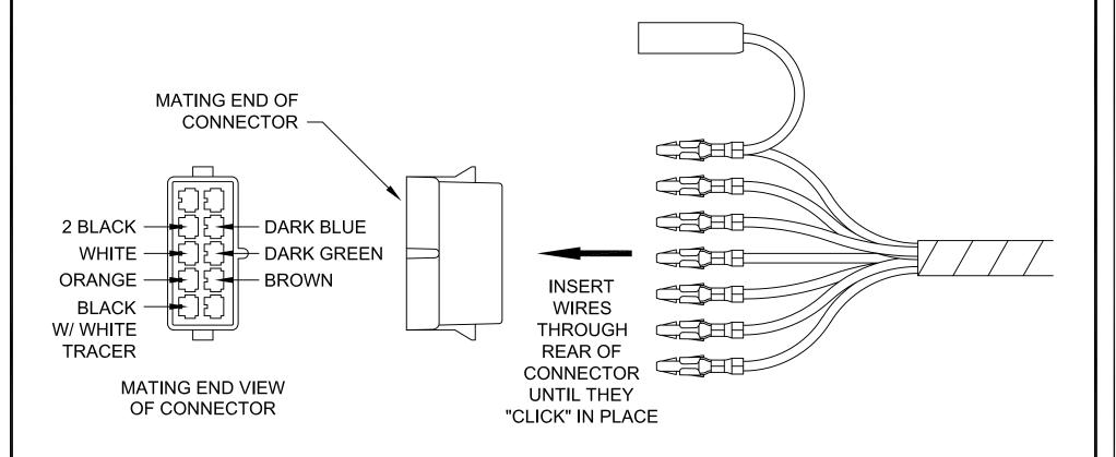
NOTE: HARNESS MUST BE INSTALLED PRIOR TO ASSEMBLING CONNECTOR TO HARNESS.
