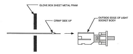
Insert a bulb into the light socket and press the assembly into the hole to lock it in sheet metal frame.
