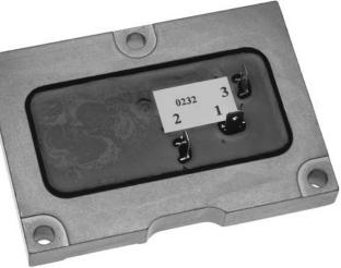
point type or aftermarket coils or M&H's own T.I. Replacement Coil. It provides output protection against failure caused by broken or disconnected plug wires, and has an extended temperature range to over 300-degrees. The state-of-the-art electronics are completely sealed in thermoplastic to keep water and contaminants out. Superior construction provides superior performance, just like all M&H Electric's products.
