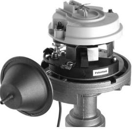
distributor. Unlike competitive systems though, no additional wires protrude from the distributor, only the original points wire. The result is a state-of-the-art ignition with an absolutely stock appearance. The Breakerless SE is so unique that it's patented !
