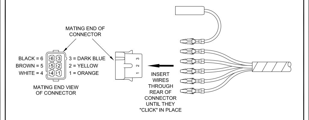
NOTE: HARNESS MUST BE INSTALLED PRIOR TO ASSEMBLING CONNECTOR TO HARNESS.
