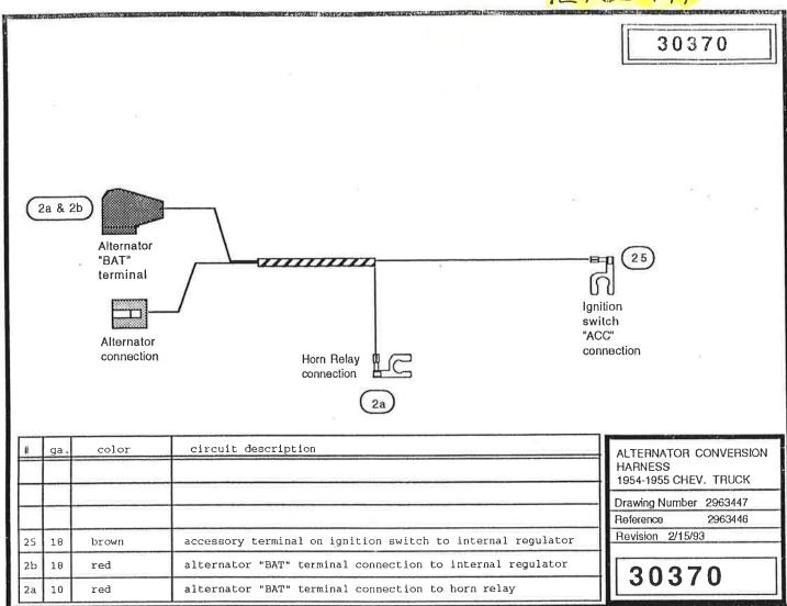
Note: This Alternator conversion is designed to work with 12 volt wiring systems only.
