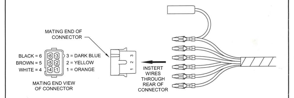
NOTE: HARNESS MUST BE INSTALLED PRIOR TO ASSEMBLING CONNECTOR TO HARNESS.
