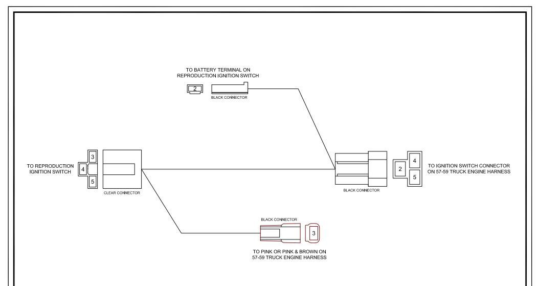
NOTE: THIS ADAPTER IS DESIGNED TO ALLOW THE 57-59 CHEVY TRUCK ENGINE HARNESSES TO BE CONNECTED TO THE REPRODUCTION IGNITION SWITCH FOR 55-56 CAR & 55-56 TRUCK.
